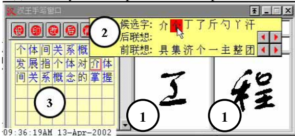
1: Handwriting area (one window per character) 2: Alternative characters selection (ACS) area (when one of characters is selected in text editing area, e.g. “介” in Figure 2, several alternative recognized characters as system recognition result will appear in this ACS area to let user select a correctly recognized character, e.g. “个” in Figure 2) 3: Text editing area (listing all of characters as recognition results) Figure 2. A user interface of a double-window spatial segmentation Chinese handwriting recognizer
