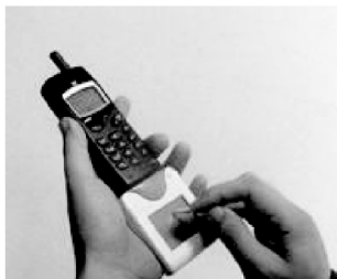
Figure 1. A mobile phone with a Chinese character handwriting recognizer. Adapted from Wu (2003).
